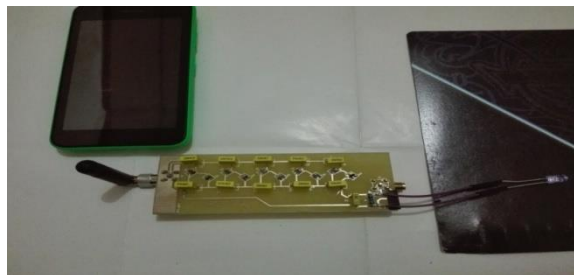
Figure 15. RFEH When the Mobile phone is Standby conditions, the LED indicator illuminates
