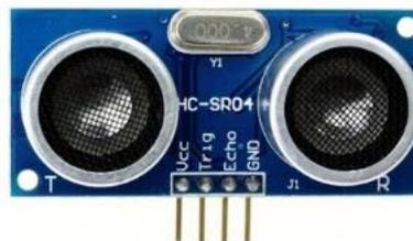
**Gambar 4.** Sensor Ultrasonik
