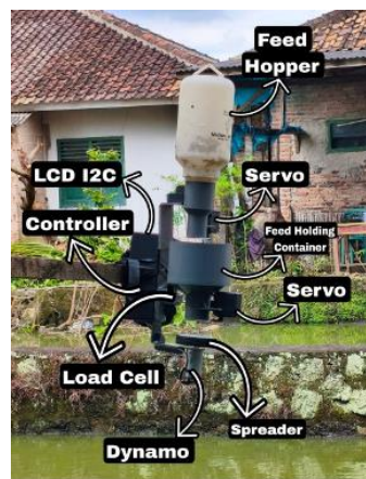
Figure 6. Portable Smart Feeder System
